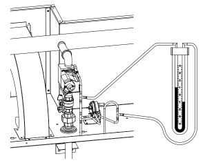
Figure 55 – Combustion Air Adjustment with a Manometer to Set Differential Pressures
